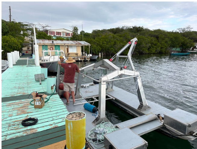
Figure 39. The seaweed farm service vessel Damisela . The Damisela was designed to fit in a shipping container for easy transport and is therefore less than 6 m long. Photo credit: Loretta Roberson, MBL.
